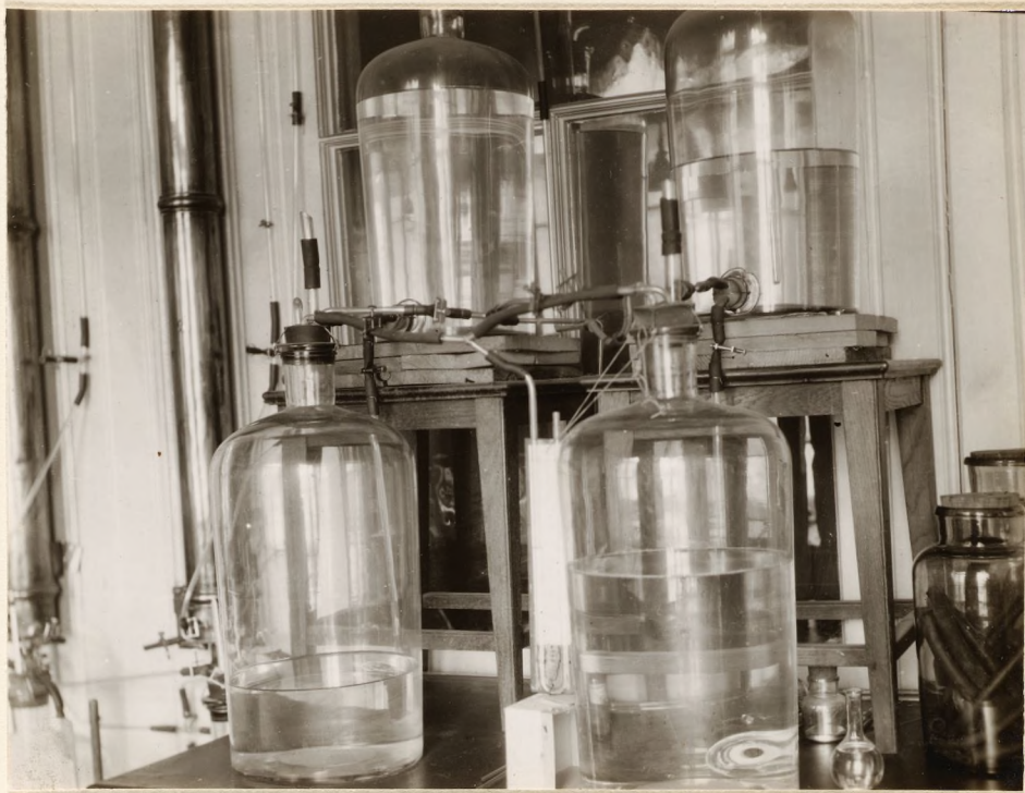
Fig. 84. System of water-levelling bottles used for the measurement of oxygen admitted to the closed-circuit apparatus of Likhatscheff in the laboratory of Kartaschefsky.
