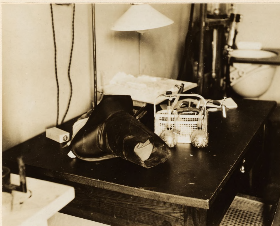
Fig. 23. The rubber neckpiece used for the Grafe head apparatus, somewhat extended so as to show the general conformation.
