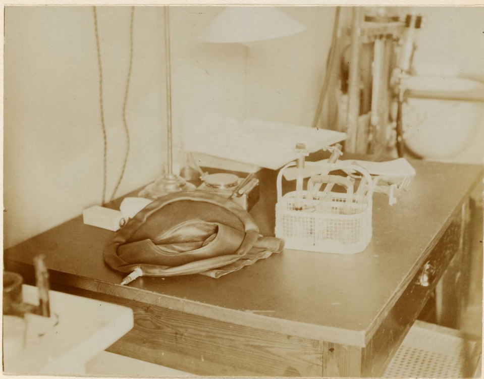
Fig. 22. Rubber collar used to connect the neck of the subject with the head apparatus of Grafe.
