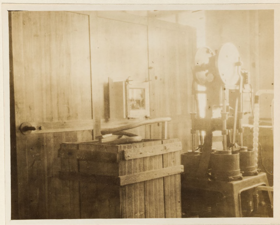
Fig. 70. Another view of the Schaternikoff respiration chamber in Moscow showing the four-cylinder pump.
