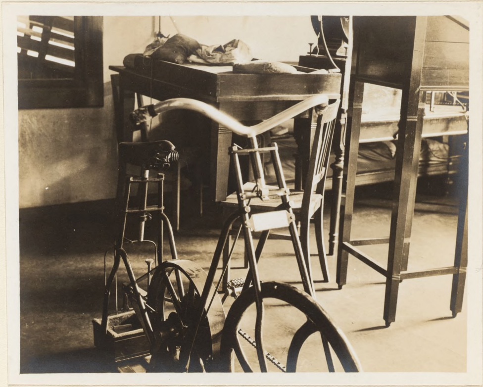
Fig. 58. Details of portions of Zuntz's new bicycle brake-ergometer in Berlin.
