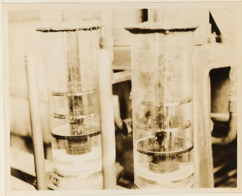
Fig. 76. Details of carbon-dioxide absorbing cylinders and valves in the Schaternikoff respiration apparatus in Moscow.
