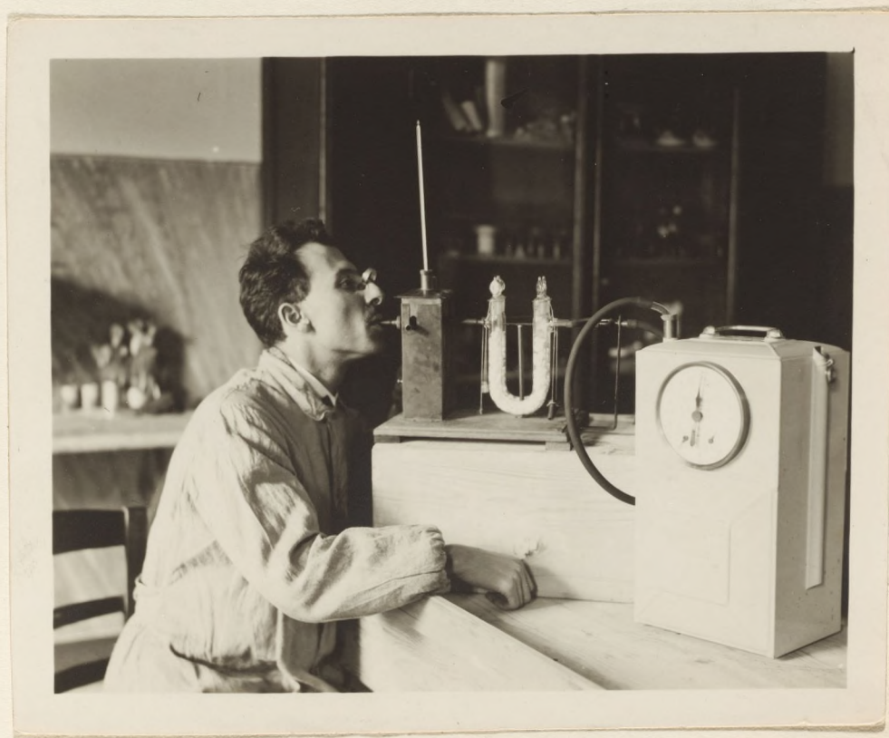
Fig. 22. Subject expiring through the Galeotti apparatus for determining the amount of moisture in the expired air.
