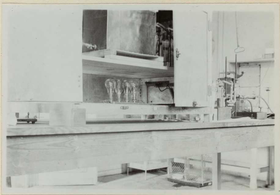
Figure 161. Strasbourg, France. University of Strasbourg, Laboratory of Physiology, Professor Kayser. Respiration chamber with electric lamps below for controlling temperature, studying rats and pigeons.
