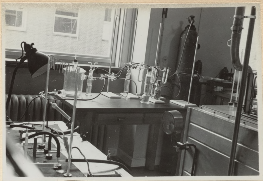
Figure 134. Heidelberg, Germany. Kaiser-Wilhelm Institut für Pathologie, Professor Krehl. Top of Rubner calorimeter, extreme left lower corner. In the right lower corner is a respiration chamber. In the rear is a small respiration chamber (Desiccator) for small animals.
