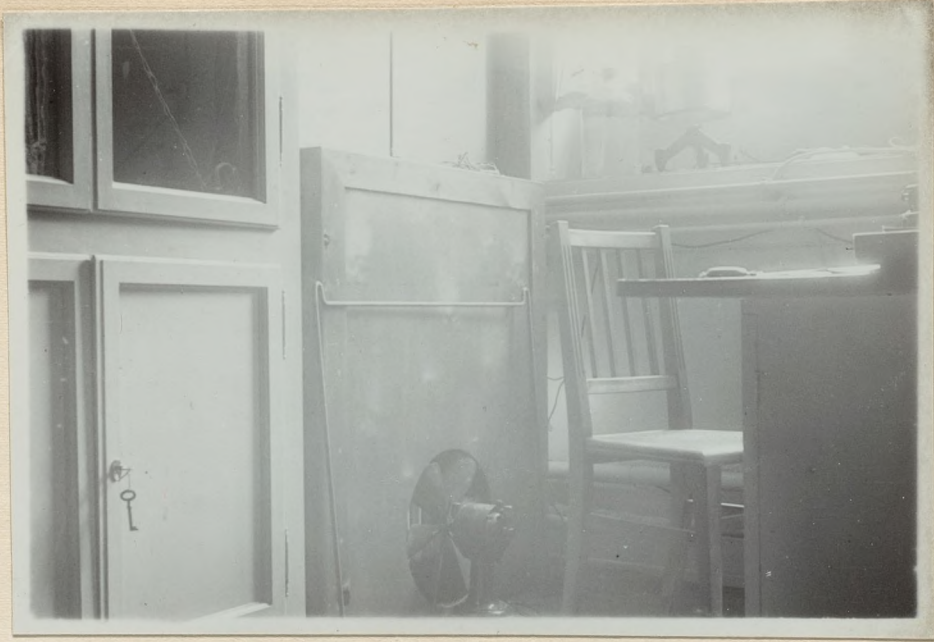
Figure 50. Copenhagen, Denmark. University of Copenhagen, Laboratory of Zoophysiology. In the center rear is the cover over the radiator for temperature regulation of the respiration room in Krogh's laboratory. Fan at bottom blows air out. The temperature is actuated by a thermostat.
