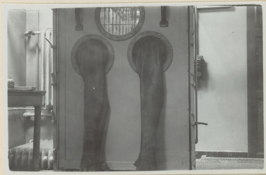
Figure 58. Copenhagen, Denmark. Agricultural Experiment Station, Department of Physiology. Closer view of rubber sleeves and window of Møllgaard's pig chamber.
