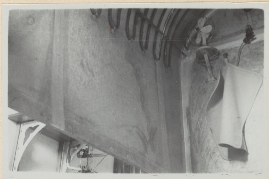
Figure 10 . Stockholm, Sweden. Carolin Institute, Laboratory of Physiology. Interior of Johansson respiration chambers, showing in the rear the temperature pipes for cooling and a rubber bag connected to the outside with a hole through the wall, allowing expansion and contraction with each respiration. It is a closed circuit and closed chamber with spirometer.
