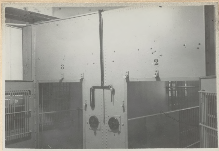
Figure 125. Leipzig-Möckern, Germany. Agricultural Institute, Professor G. Fingerling. Double respiration chamber for two animals.
