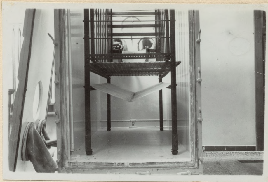
Figure 55. Copenhagen, Denmark. Agricultural Experiment Station, Department of Physiology. Møllgaard's respiration chamber for swine, showing long rubber gloves at front and rear for handling feces, excreta, and feed.
