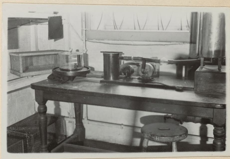
Figure 70. Edinburgh, Scotland. University of Edinburgh, Department of Physiology, Laboratory of Sir Edward Sharpey-Schafer. Schafer's metabolism apparatus for rats. Small bell jar with essentially the same equipment for soda-lime as the cat apparatus. The Sadd valve leads off to the right to the spirometer.
