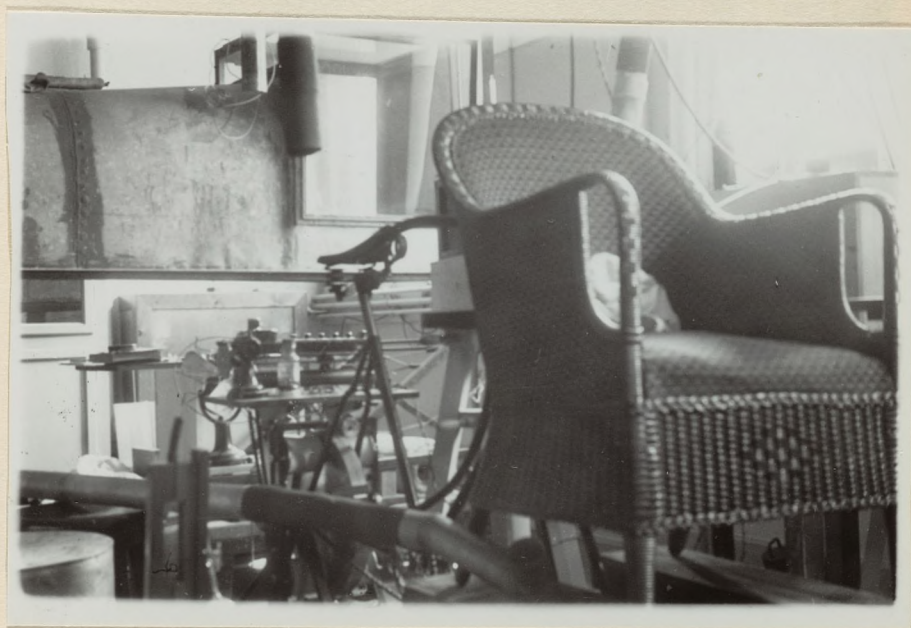
Figure 40. Copenhagen, Denmark. University of Copenhagen, Laboratory of Zoophysiology. Krogh apparatus. Chair used by subject while resting before riding. In the background one sees the seat of the bicycle ergometer, and at the left the cover of a cot calorimeter; in the foreground at the lower left, the air pipe with the mercury sampler for the Eskimo sampling device.
