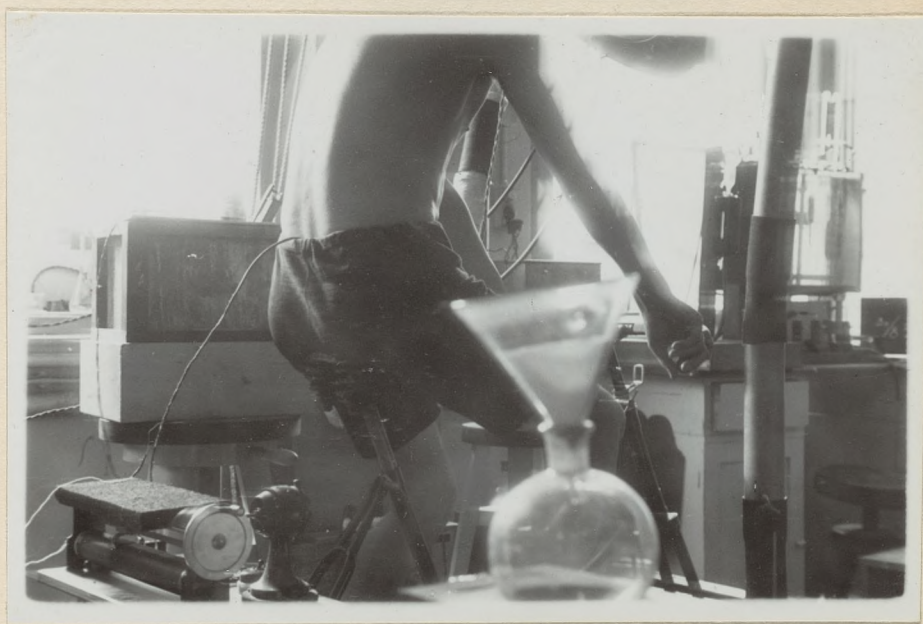
Figure 44 . Copenhagen, Denmark. University of Copenhagen, Laboratory of Zoophysiology. Krogh's subject on bicycle ergometer, stripped to the waist. Thermometer leads for rectal temperature seen coming out of trousers. Electrical method for controlling ergometer load at the lower left-hand corner.
