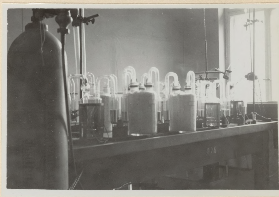
Figure 124. Leipzig, Germany. University of Leipzig, Physiological-Chemical Institute. Absorbing train for Karl Thomas' respiration apparatus, showing bottles connected by mercury seals.
