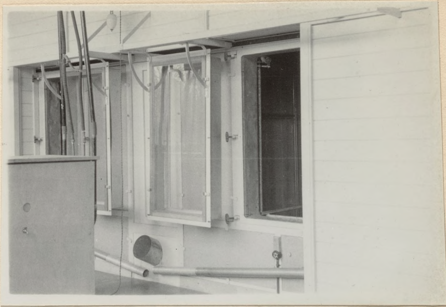
Figure 91 . Utrecht, Holland. Physiological Institute. Double door entrance to Noyons' electric compensation calorimeter. The door at the right is where the patient is put in on the bed.
